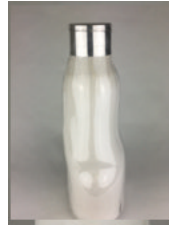
3 Blister form Plastic and/or laminate Socket
